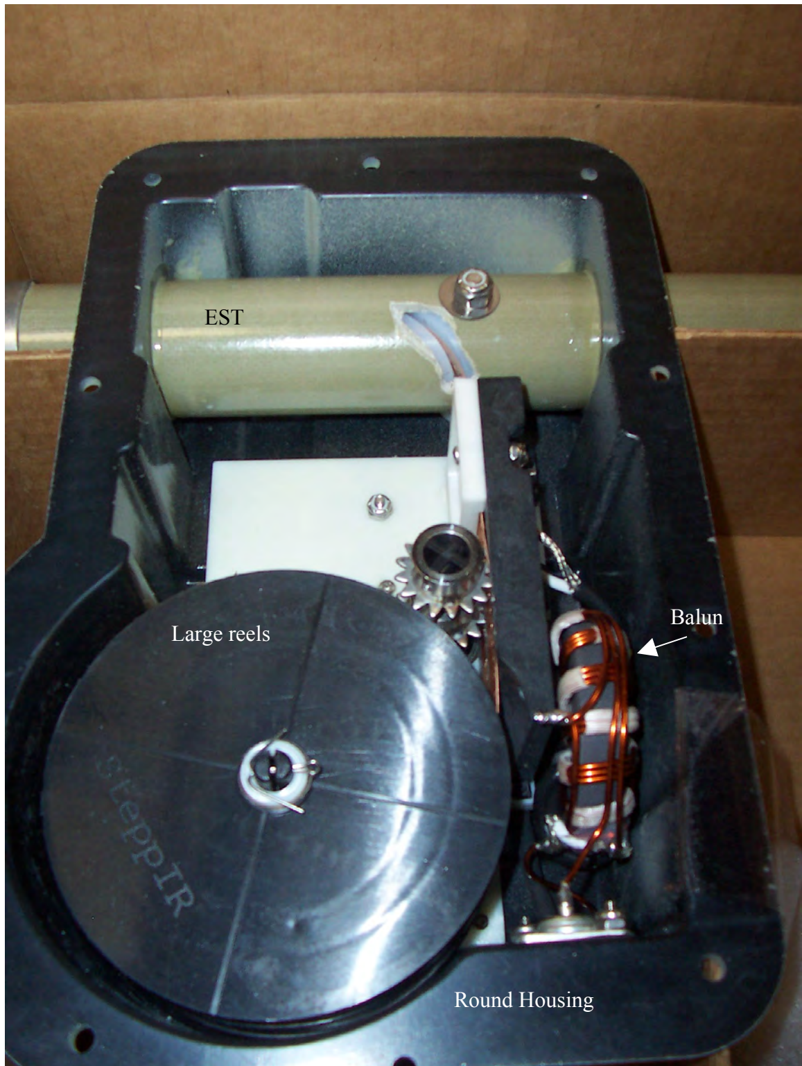
Figure 4-7 - 30/40 Driven - round housing has big reels inside and has balun
