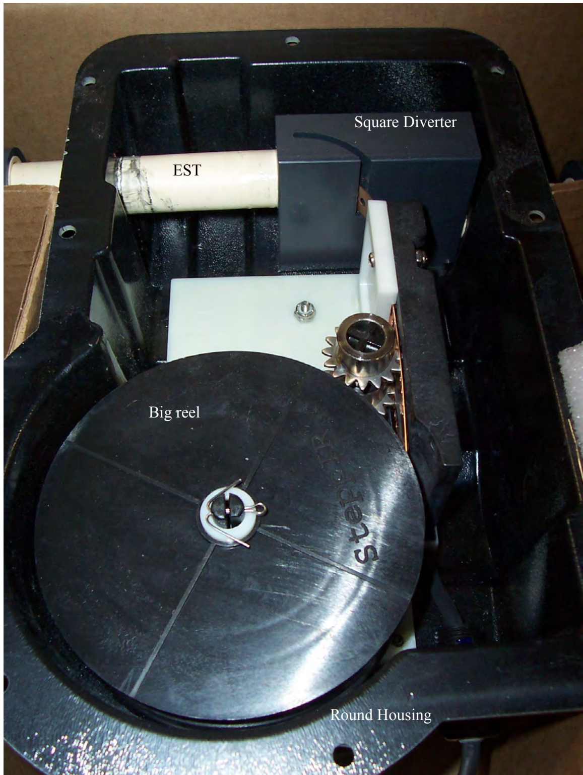
Figure 4-9 - MonstIR 40m Passive Director & Reflector - have round housings, big reels, and no baluns
