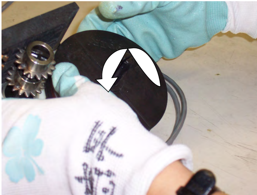
Figure #2-2 - Copper reel winding procedure
