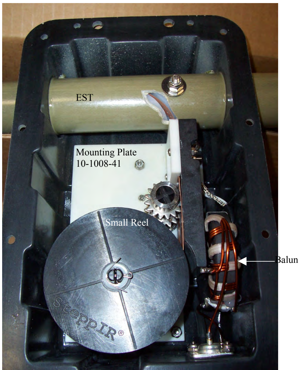
Figure #4-6 - Driven housing - interior view has a rectangular and also has a balun
