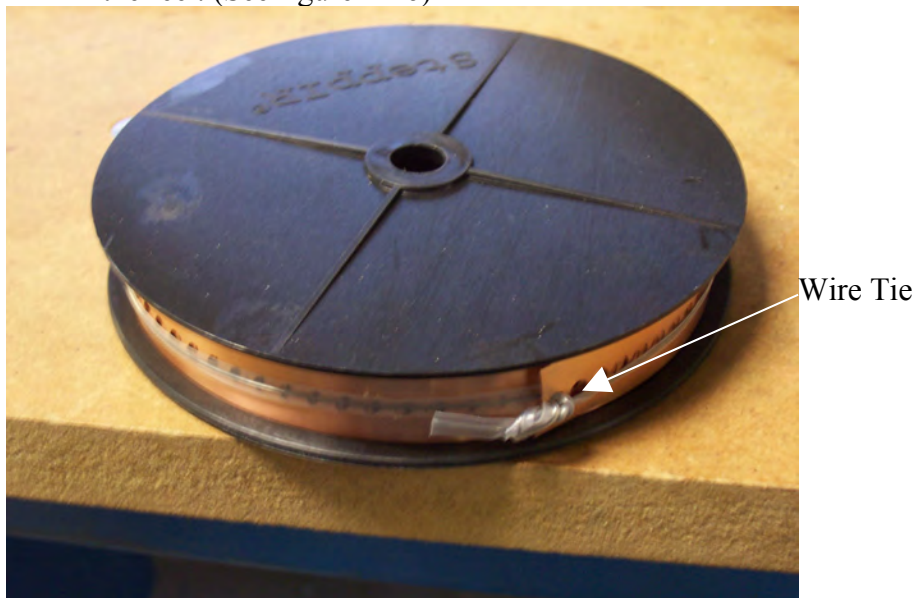
Figure # 1-6 - Reel loaded with Copper with wire tie on it
